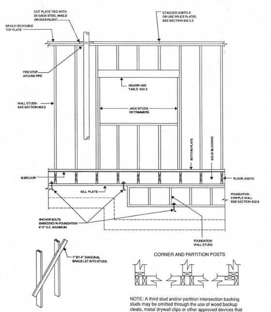
will serve as an adequate backing for the facing materials. Apply approved sheathing or brace exterior walls with 1" by 4" braces let into studs and plates and extending from bottom plate to top plate. See Section 602.9.
